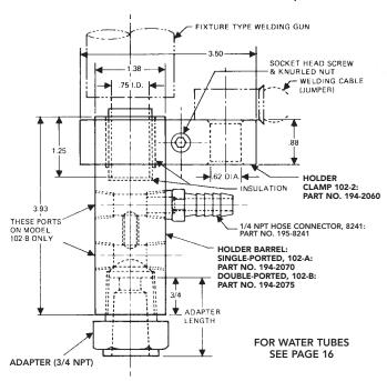
To determine distance adapter sticks out from holder deduct 3/4" from length of adapter selected. Water tubes 3/4" longer than adapter will install approximately flush with adapter face.
