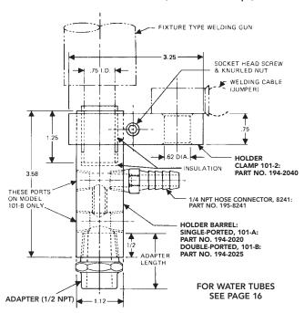
To determine distance adapter sticks out from holder, deduct 1/2" from length of adapter selected. Water tubes 1/2" longer than adapter will install approximately flush with adapter face.
